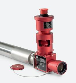
Boresighting a MBT or IFV may be hard to do due to the height of the main gun. The Nedinsco BORCAM camera module can be mounted to our boresights, to allow the gunner to align the gun with the weapon's optical sensors from within the turret. A safe and efficient option, shortening the alignment time, reducing the number of people, and enhancing alignment accuracy by using a monitor.
